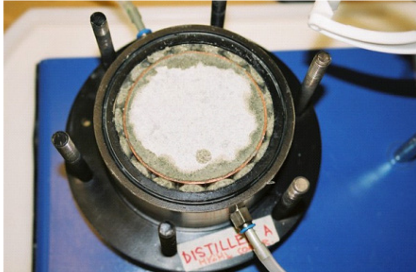
Figure 3-12. Growth of soft clay through the perforation of a copper tube confining a dense MX-80 clay core in an 80 mm diameter oedometer. Appearance at removal of the lid 8 hours after start. The larger part of the core is still unaffected by water.
