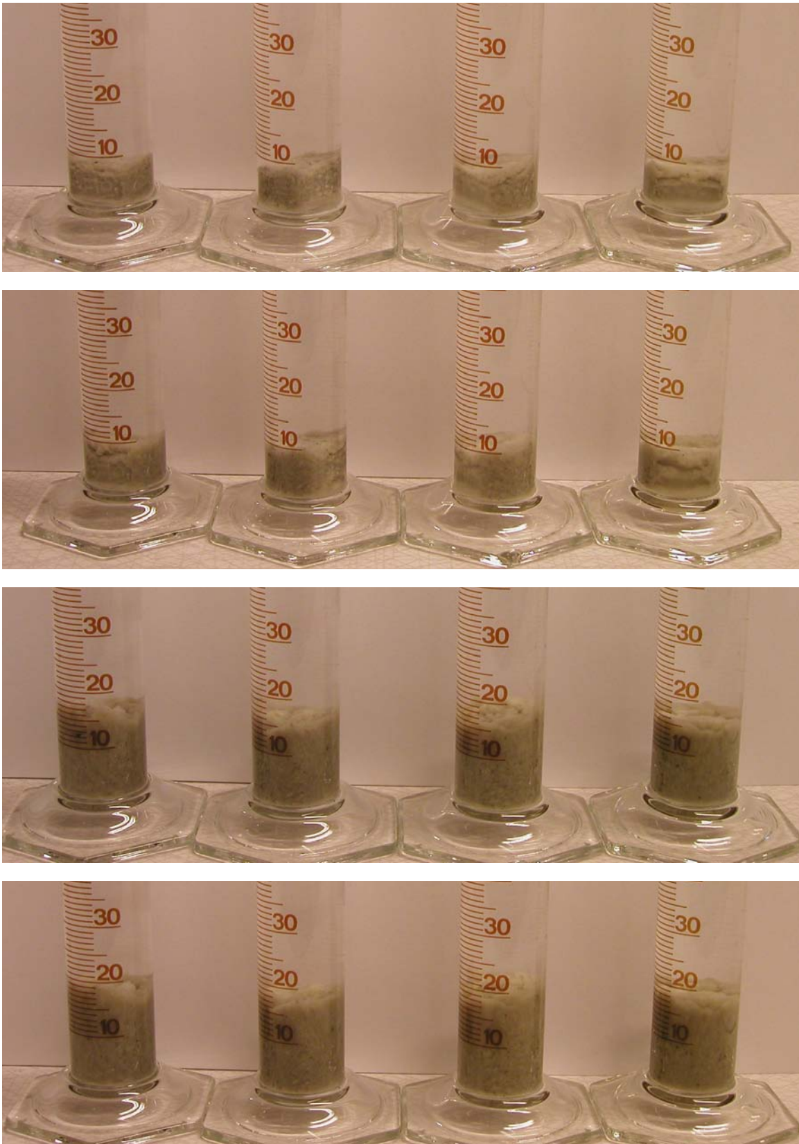
Figure 1-14. Pictures showing the swelling capacity of four materials. From left: w=10\% 100 MPa, w=10\% 300 MPa, w=2.5\% 100 MPa, w=2.5\% 300 MPa. The upper picture shows the result after 5 min, next picture after 1 hour, next 24 hours and the lower after 48 hours.
