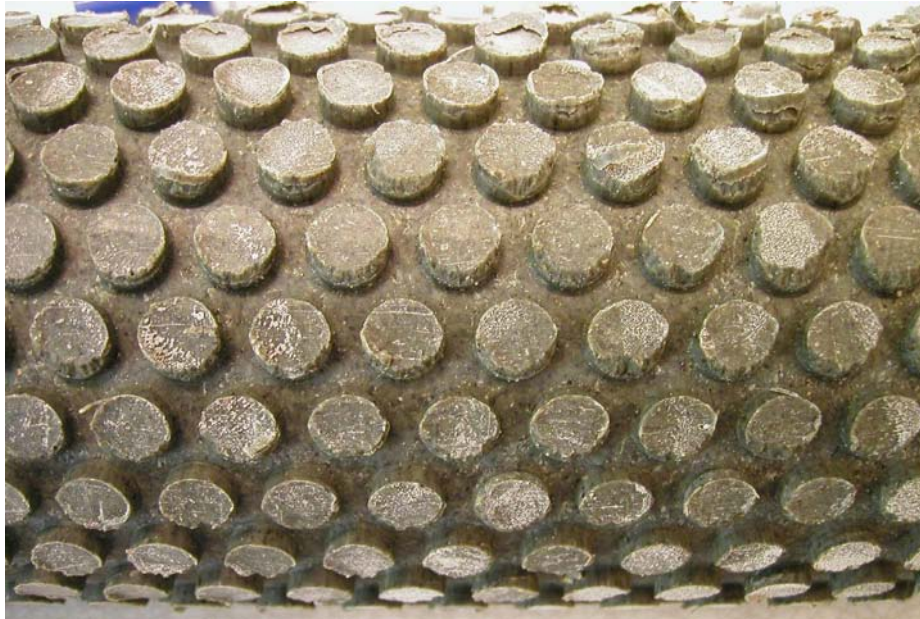
Figure 4-20 Picture showing the clay sample after dismantling of the copper tube. The clay from the holes is still solid and this facilitated the sampling.
