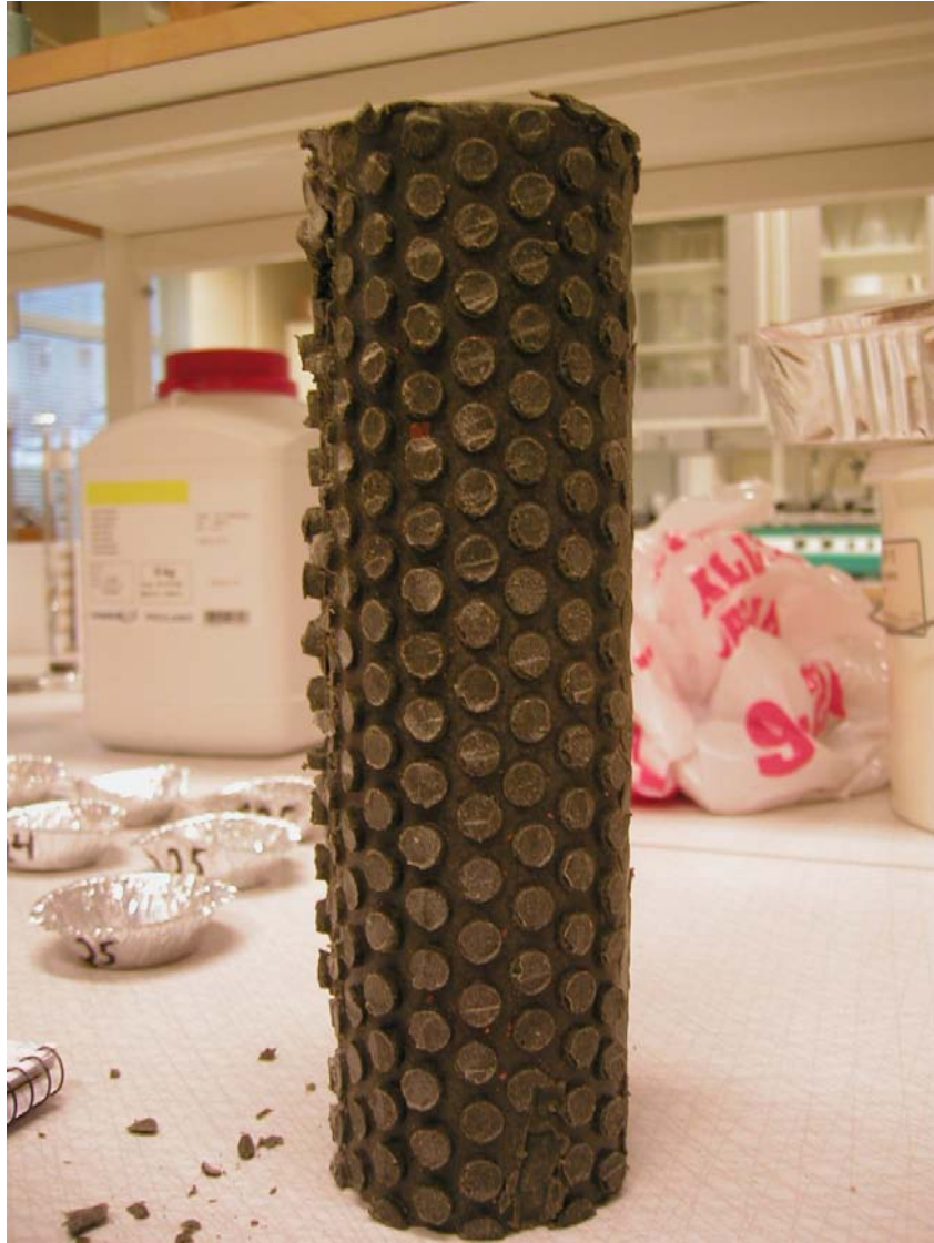
Figure 1-7. Picture showing the clay sample after dismantling of the copper tube. The clay from the holes is still solid and this facilitated the sampling.
