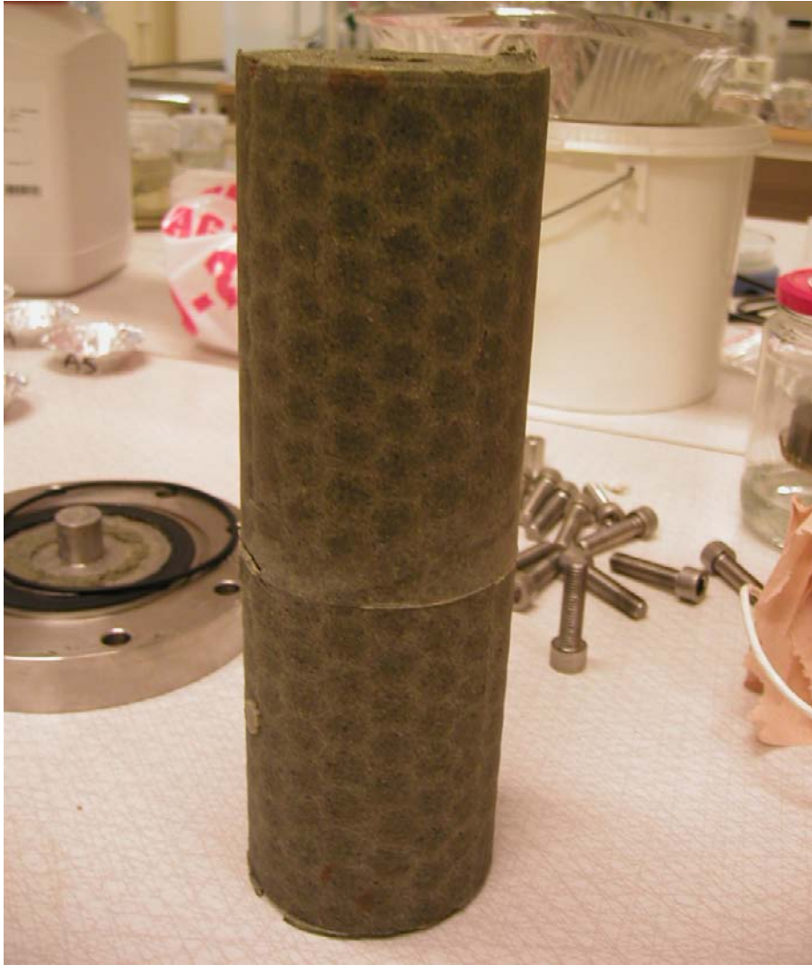
Figure 1-6. Picture showing one of the samples immediately after dismantling. It was possible to see the pattern from the perforated tubes in the clay surface. Both samples looked very similar.
