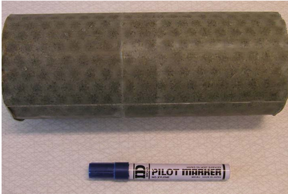
Figure 4-18 Picture showing the sample saturated with distilled water immediately after dismantling. It was possible to see the pattern from the perforated tubes in the clay surface. Both samples looked very similar.
