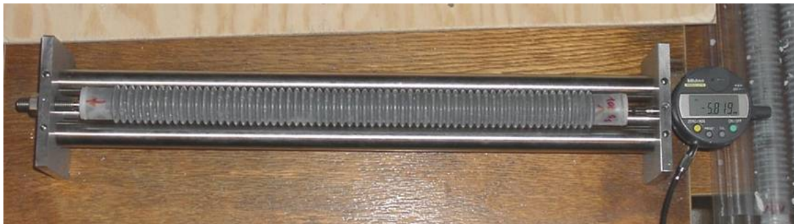
Figure 2; Flexible tube for autogenous shrinkage.
