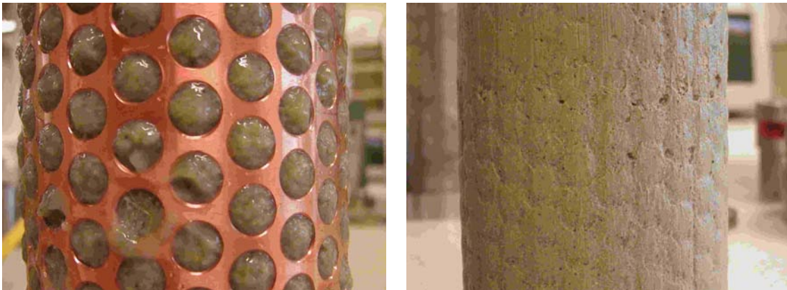
Figure 4-9. Pictures taken after interruption of the 1 hour tests. The left picture shows the sample which has been surrounded by distilled water and the right shows the sample which has been surrounded by 3.5% \text{CaCl}_2 water. The water ratio of the clay outside the copper was for this sample about 118%.
