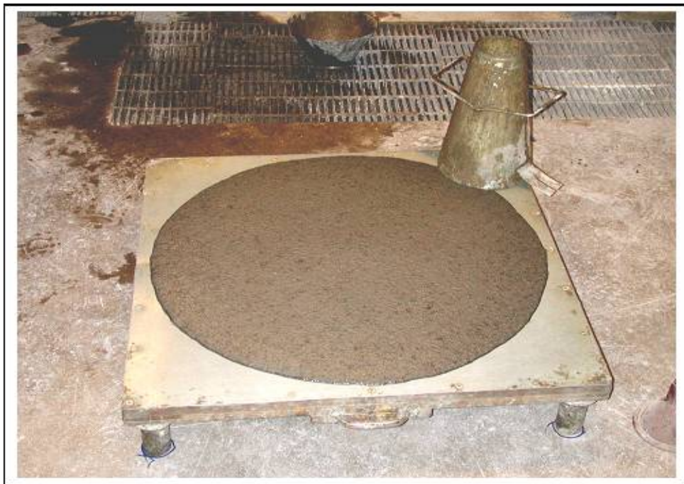
Figure 1; Picture of flow for the borehole plug concrete. This concrete is self-compacting in a borehole.
